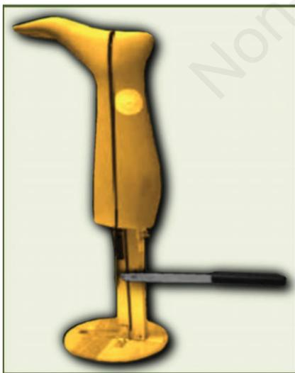
**Figure 5.** The mannequin leg with the lever arm, which when pushed down, guarantees a 1 cm enlargement in circumference (device number 14).
