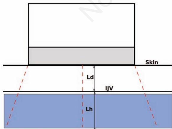
Figure 1. Schematic representation of an ultrasound probe insonating an internal jugular vein (IJV) in the L plane. The IJV's walls are represented. The distance  $Ld$  between the IJV and the skin and the wall distance  $Lh$  of the IJV are shown.
