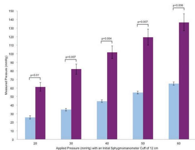
**Figure 3. Differences between measured pressures by an air-bladder sensor based on placement underneath the airbag or fabric of a sphygmomanometer (diameter: 12 cm).** Across all applied pressures (20 mmHg to 60 mmHg) for a cuff of an initial diameter of 12 cm, PicoPress displayed significantly higher pressures when placed underneath the cuff fabric. This result was statistically significant ( $P<0.05$ ) for all applied pressures.
