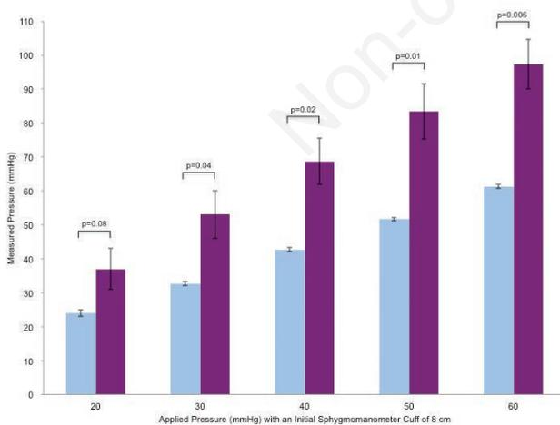
**Figure 2. Differences between measured pressures by an air-bladder sensor based on placement underneath the airbag or fabric of a sphygmomanometer (diameter: 8 cm).** Across all applied pressures (20 mmHg to 60 mmHg) for a cuff of an initial diameter of 8 cm, PicoPress displayed significantly higher pressures when placed underneath the cuff fabric. This result was statistically significant ( $P<0.05$ ) for all applied pressures except 20 mmHg.
