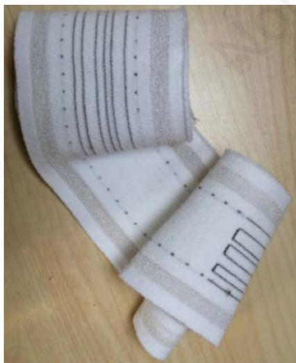
**Figure 1. Functional prototype Smart Bandage showing three transducers knitted into a compression bandage.**
