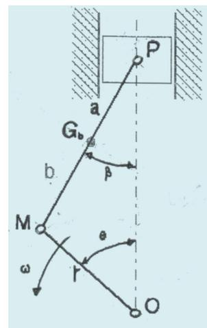
The system made up of three parts connected one to each other by three rotoidal couples and by a prismatic
