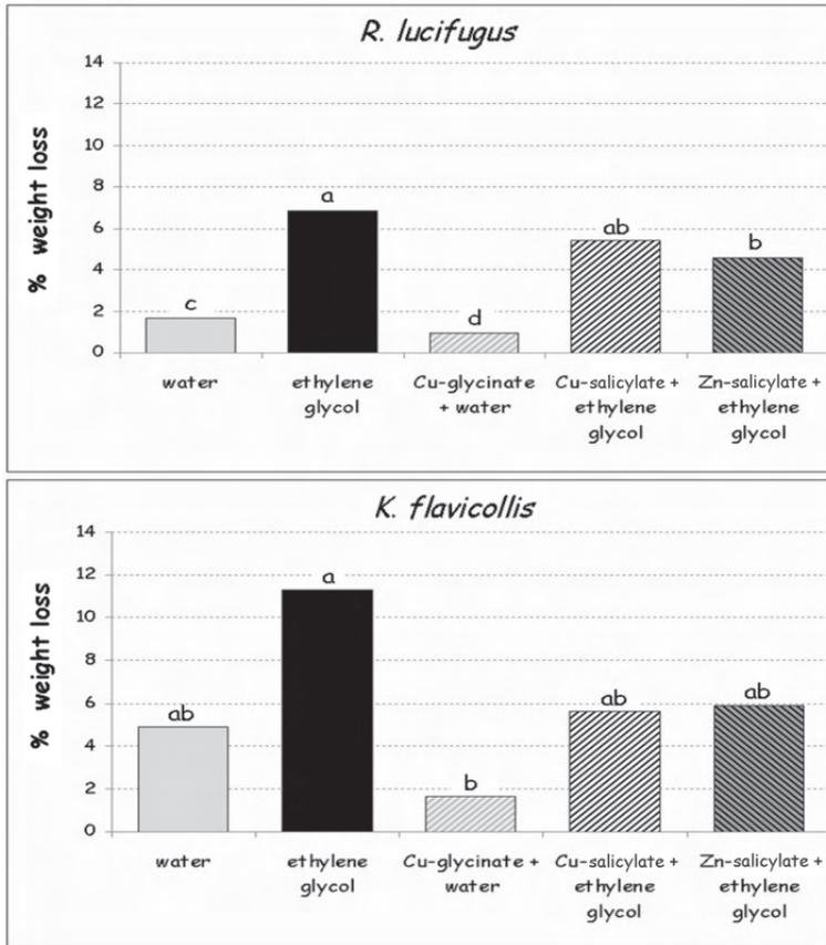
Fig. 2 - Test 2, weight loss (%) due to *R. lucifugus* (above) and *K. flavicollis* (below) consumption on differently treated wood slices, recorded at the end of the experiments. Columns indicated by different letters show significant differences at the Tukey test ( $p \leq 0.05$ ).
