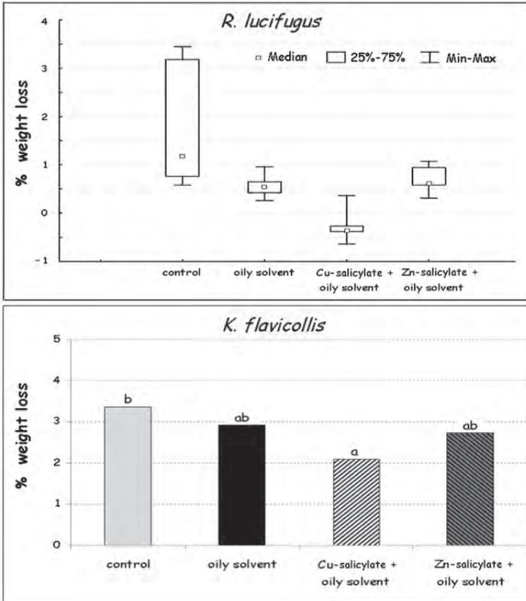
Fig. 1 - Test 1, weight loss (%) consumption on differently treated wood slices, recorded at the end of the experiment due to the two species. *R. lucifugus* data (above) were processed using non parametric Kruskal-Wallis analyses of variance. *K. flavicollis* data (below) were processed using Tukey test to separate the media ( $p \leq 0.05$ ). Columns indicated by different letters show significant differences.
