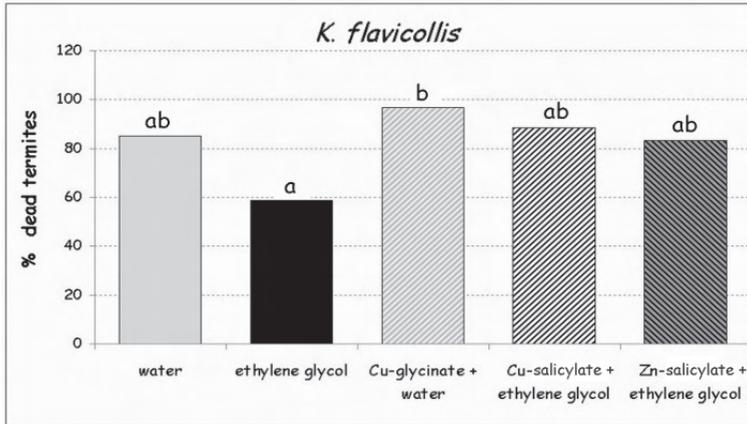
Fig. - Test 2, *K. flavicollis* average percentage of mortality in differently treated wood slices, recorded at the end of the experiment (90 d). Columns indicated by different letters show significant differences at the Tukey test ( $p \leq 0.05$ ).
