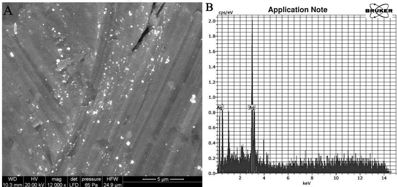
Figure 2. A and B) Scanning electron microscopy and energy dispersive X-ray image of AgNPs synthesized from *E. milii*.
