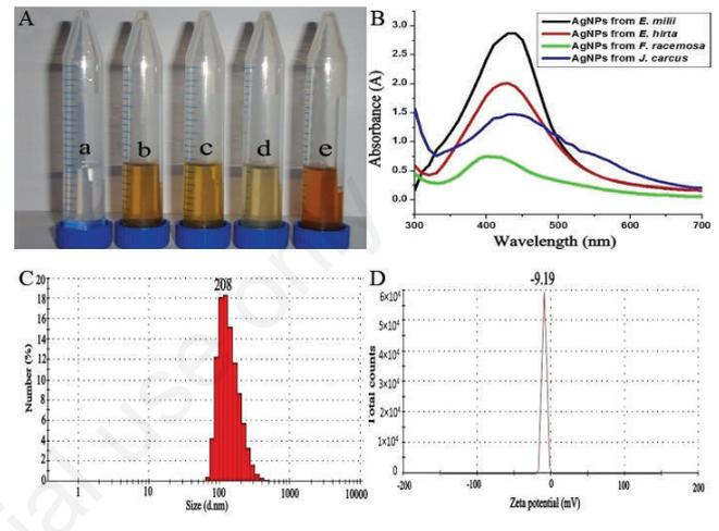
Figure 1. A) Tubes showing colour change of AgNPs: a. silver nitrate solution, b. *E. milii*, c. *E. hirta*, d. *F. Racemosa*, and e. *J. curcas*. B) UV spectra of AgNPs. C and D) Particle size and zeta potential analysis of AgNPs produced from *E. milii* latex.
