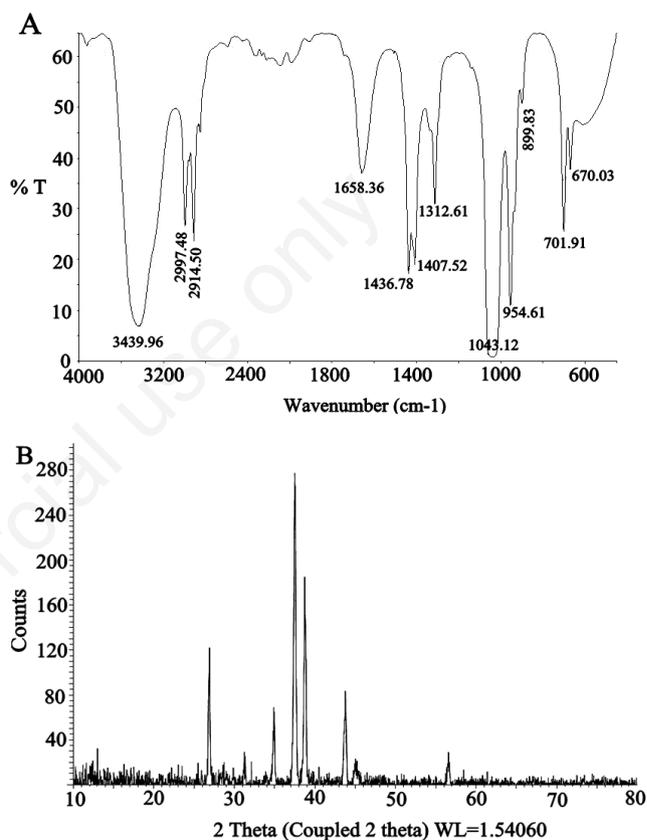
Figure 3. A and B) Fourier transformed infrared spectroscopy and X-ray diffraction spectrum of AgNPs synthesized from *E. milii*.
