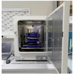
Figure 1. Random Positioning Machine (RPM).The RPM (Dutch Space, Leiden, Netherlands) (a) was run in a commercially available incubator at 34°C and 5% CO<sub>2</sub> (b).
