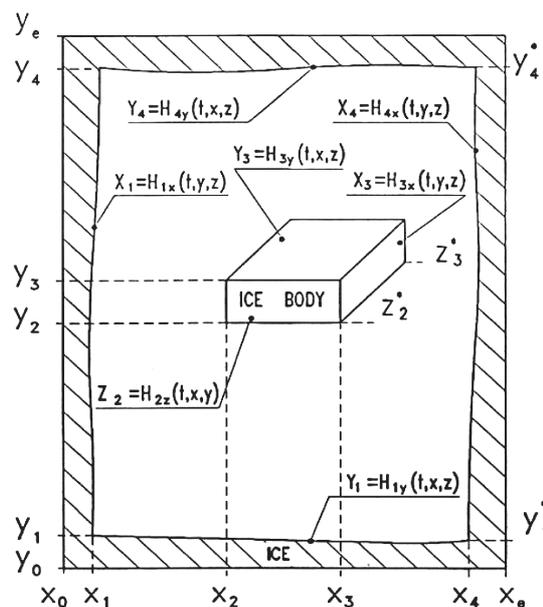
Fig. 2 - Diagram of the conservation cell and ice body.
