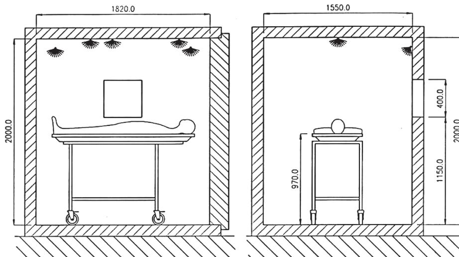
Fig. 1 - Low temperature conservation cell ( $-6^{\circ}\text{C}$ ) with controlled humidity.
