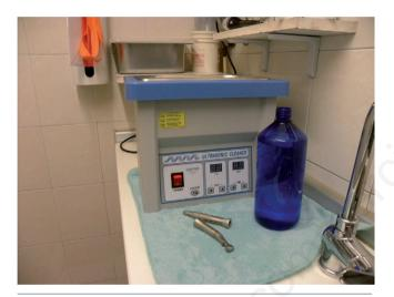
Figure 4. Picture of ultrasonic washing machine.
