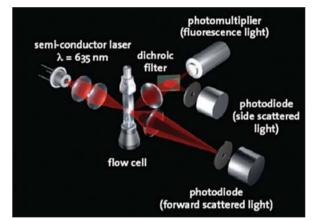
Figure II. The Optical unit of UF-1000i analyzer.
