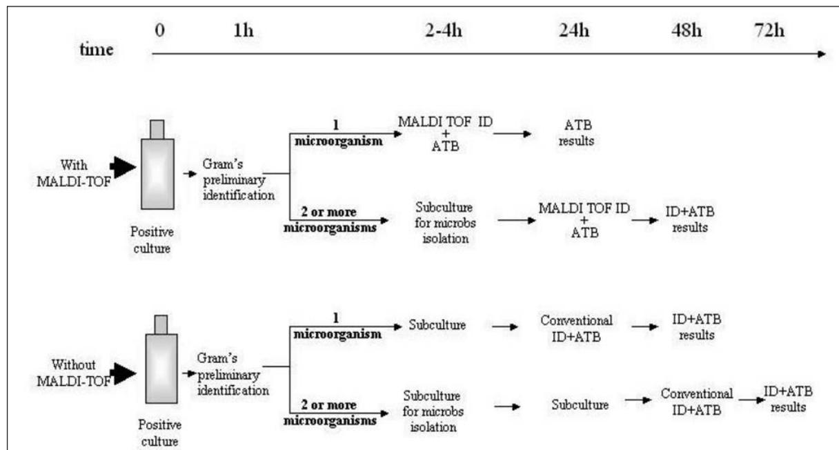
**Figure II.** Time course comparison for the characterisation of microorganisms in a positive blood culture with and without MALDI-TOF MS. ATB= antibiogram, ID= identification
