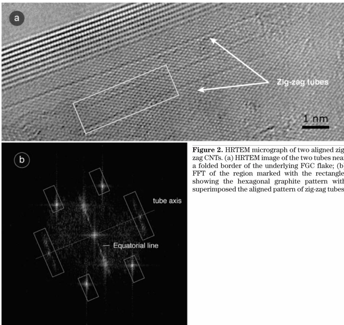
**Figure 2.** HRTEM micrograph of two aligned zig-zag CNTs. (a) HRTEM image of the two tubes near a folded border of the underlying FGC flake; (b) FFT of the region marked with the rectangle, showing the hexagonal graphite pattern with superimposed the aligned pattern of zig-zag tubes.
