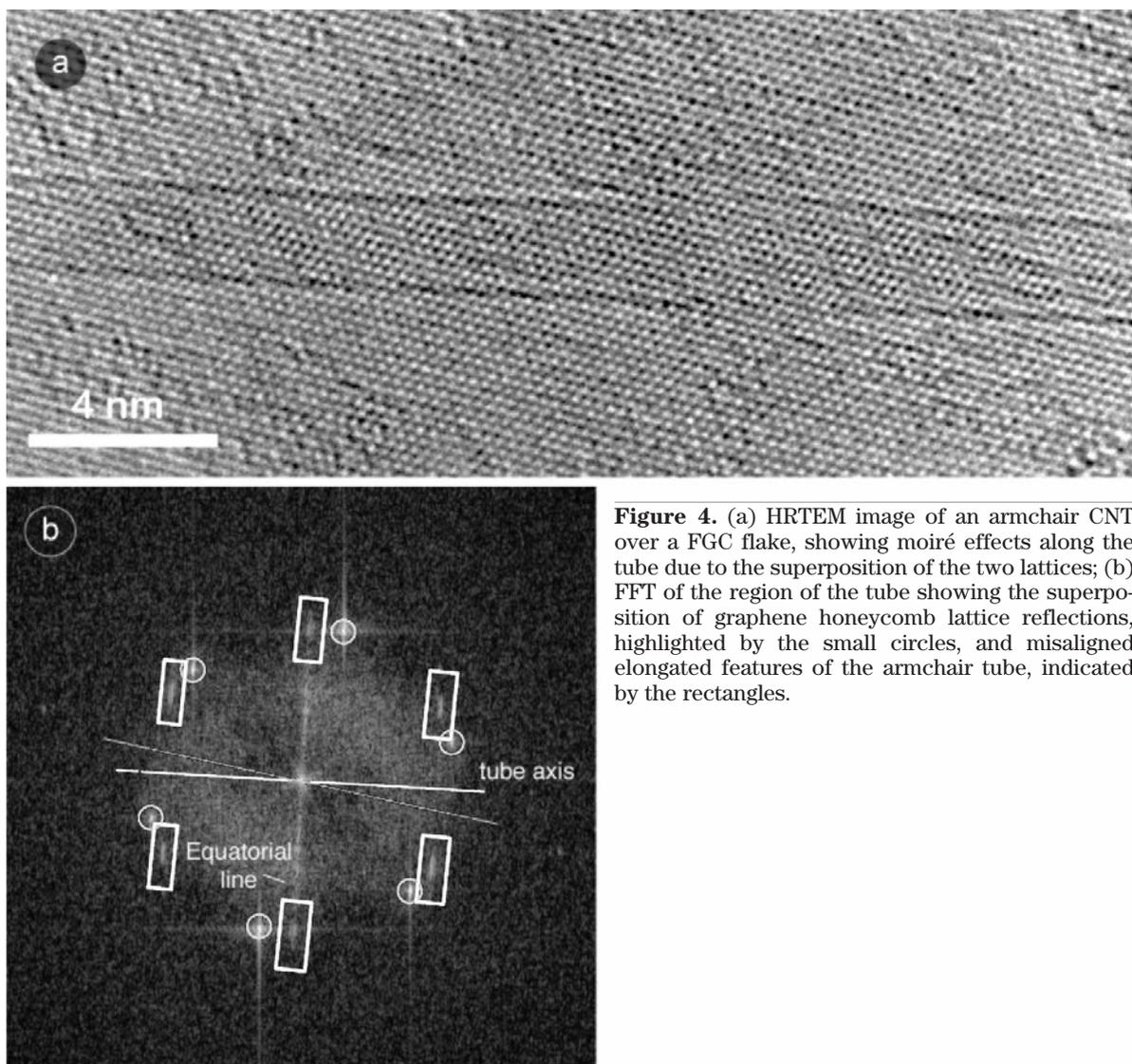
**Figure 4.** (a) HRTEM image of an armchair CNT over a FGC flake, showing moiré effects along the tube due to the superposition of the two lattices; (b) FFT of the region of the tube showing the superposition of graphene honeycomb lattice reflections, highlighted by the small circles, and misaligned elongated features of the armchair tube, indicated by the rectangles.
