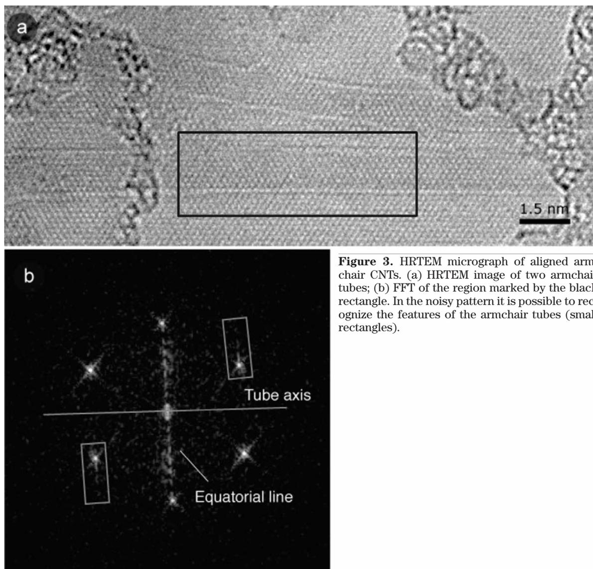
**Figure 3.** HRTEM micrograph of aligned armchair CNTs. (a) HRTEM image of two armchair tubes; (b) FFT of the region marked by the black rectangle. In the noisy pattern it is possible to recognize the features of the armchair tubes (small rectangles).
