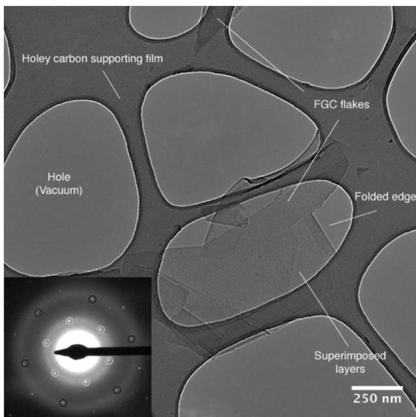
**Figure 1.** TEM image of the produced thin FGC flakes. In the image a flake is suspended over the amorphous carbon support of the TEM grid. (Inset) Electron diffraction pattern from the central area of the flake, showing graphite hexagonal symmetry, highlighted by black and gray circles.
