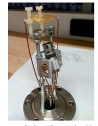
**Figure 13.** Homemade channeltron and Golden Woven Mesh holder lodged in a feedthrough flange (maximum current 10 A) for the vacuum chamber.
