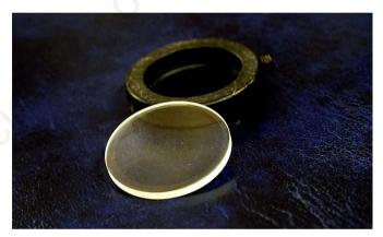
**Figure 1.** Picture of the 300 nm thickness nanoporous alumina sample. It is clearly visible a blueish layer corresponding to the deposited alumina.
