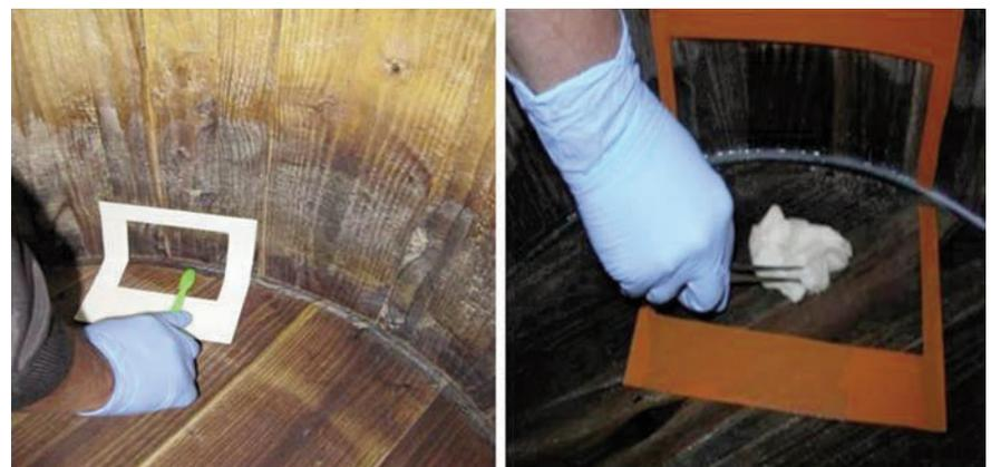
**Figure 2. Sampling on the wooden vat surfaces.**
