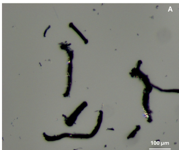
Figure 1. PET MFs under optical microscope (A) and their FTIR spectrum (B).
