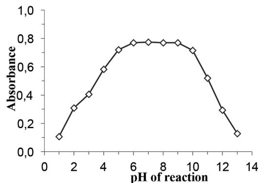
**Figure 2.** The complex absorbance at various reaction pH at a Hg concentration of 1.0 µg/L in water.
