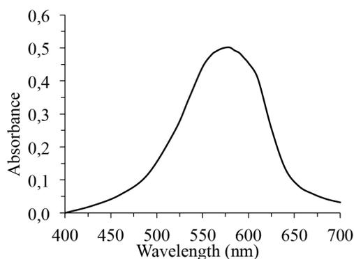
**Figure 1.** Wavelength spectra of reaction product complexes in PVC-DOS-based optical membranes.
