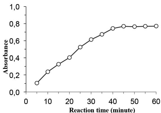
**Figure 3.** At a Hg concentration of  $1.0 \mu\text{g/L}$ , membrane response time and absorbance were measured.
