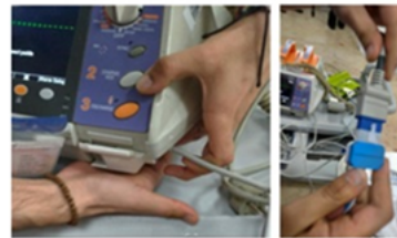
IV. remove defibrillator paddle connection, insert pad connection.
