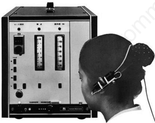
Figure 2. The first pulse oximeter, OLV-5100, patented by Takuo Aoyagi and produced by Nihon Kohden in 1974. Freely available from the internet.
