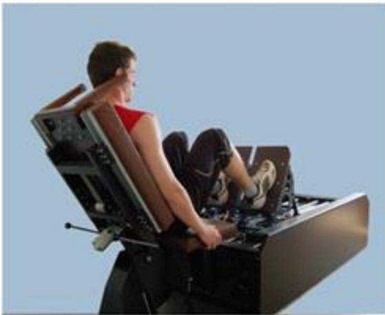
**Fig 3.** Universal computer controlled linear motor based leg press dynamometer.
