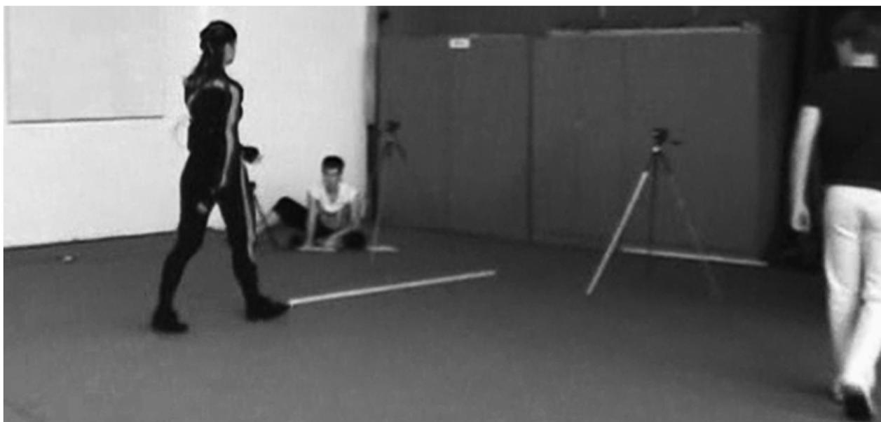
**Fig 1.** Measurement set-up: (i) a subject in the MOV dress that wirelessly transfers the data to the computer which was operated by the first measurer, (ii) the sitting measurer was noting down the time acquired by the photocells and made additional precise measurements of the last remaining step using the measurement tape, (iii) the third measurer was only estimating the length of the last step and measuring the time with the manual stop-watch.
