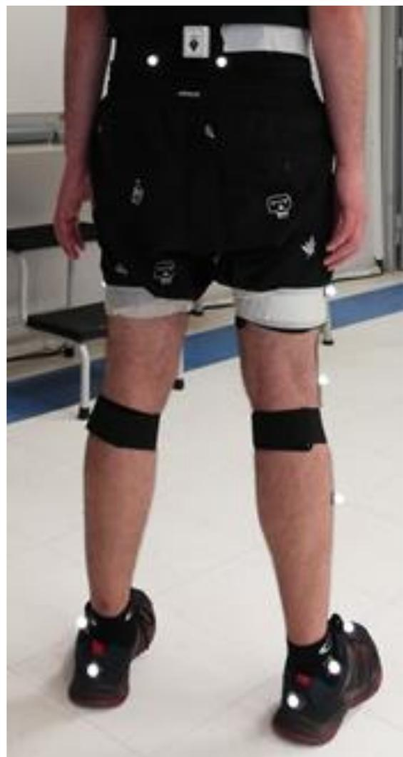
**Fig 2.** Location of the IMU and the markers using the VICON "Plug-In-Gait" lower body kinematic model.
