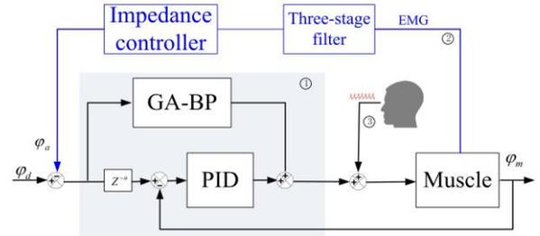
**Fig 2.** The whole framework of our cooperative controller. It consisted of a FES controller and an impedance controller. The FES controller was composed of a GA-BP networkbased feedforward controller and a PID-based feedback controller. A three-stage filter was designed to extract volitional force/torque from raw EMG. 1: FES controller, 2: impedance controller, 3: voluntary contribution.
