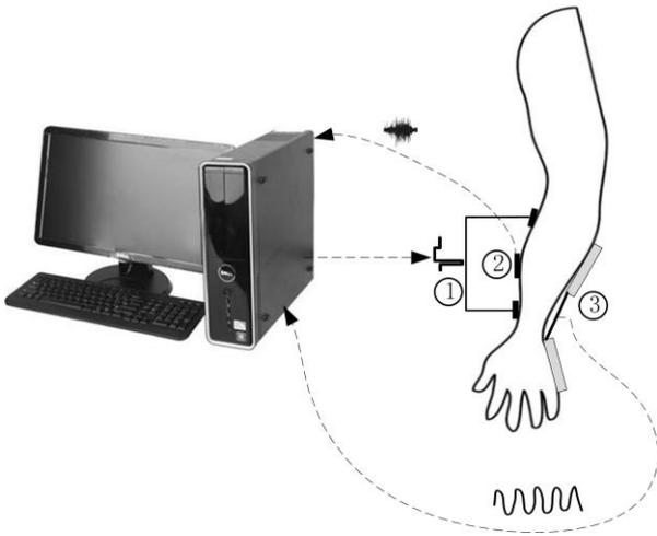
**Fig 1.** The experimental setup of our study. The EMG and angle of wrist was fed into computer. The controller in computer would then send commands to a FES device. The FES device exerted electrical stimulation on the targeted muscle. 1: FES electrodes, 2: EMG electrode, 3: goniometer.
