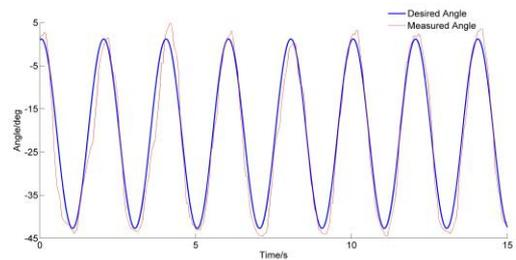
**Fig 3.** The tracking performance for FES controller alone.
