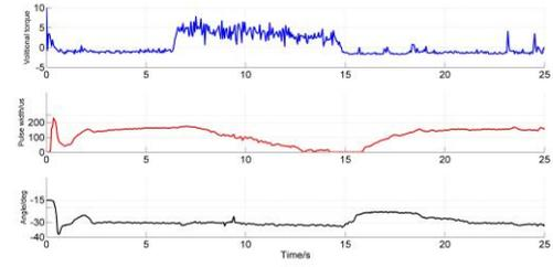
**Fig 5.** The performance of cooperative controller. These subplots show the waveforms of volitional torque, pulse width of FES, and angle of wrist, respectively.
