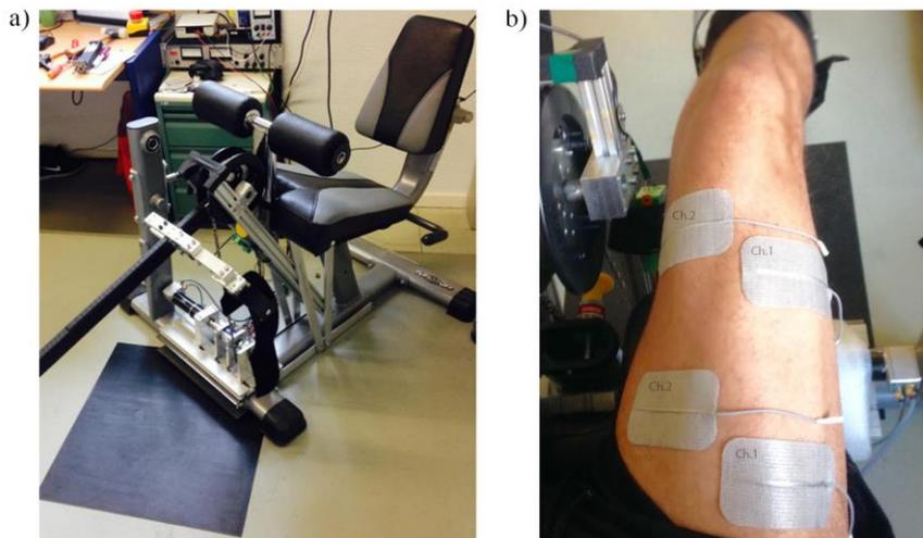
**Fig 1.** (a) The Knee Dynamometer designed to measure isokinetic knee joint torque.
