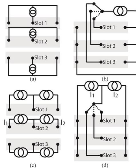
Fig 2 Stimulator configuration for a three slot book - (a) Independent between slots, Paired, anodes (IP); (b) Common between slots, Paired, anodes (CP); (c) Independent between slots, UnPaired, anodes (I\|P); (d)
