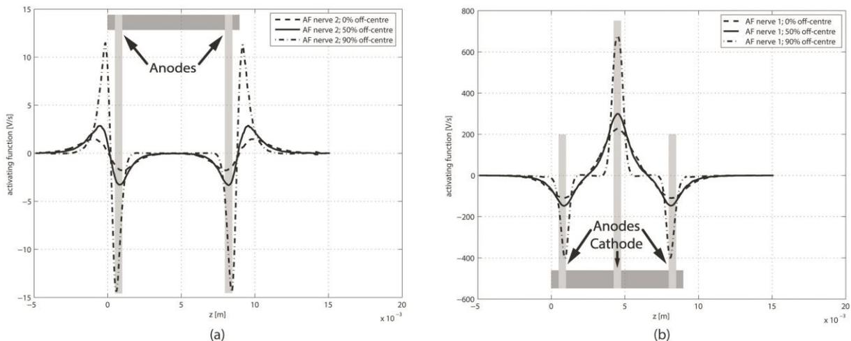
**Fig 5.** Activating function for nerve fibres at 3 locations inside a nerve. (a) Nerve in active slot. (b) Nerve in peripheral, non-stimulating, slot.
