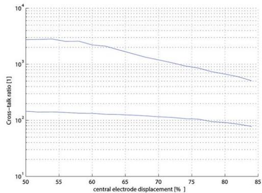
**Fig 8.** Comparison of cross-talk ratio for electrode displacement for IP (upper curve) and CP (lower curve).
