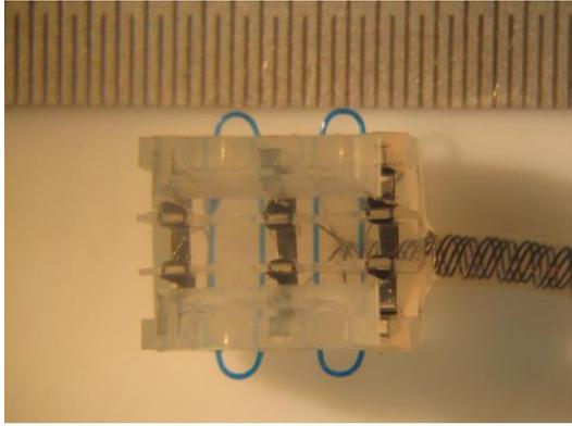
Fig 1. LARSI stimulator with three slot of tripoles. Reproduced with permission.<sup>3</sup>
