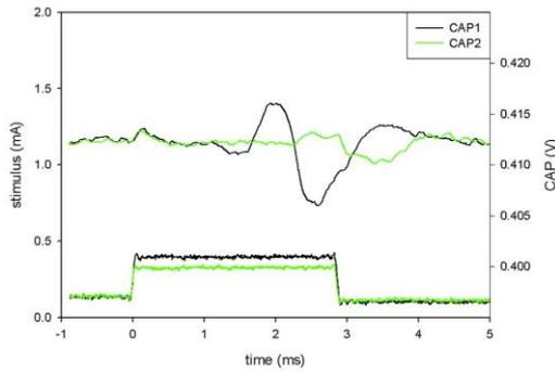
**Fig 6.** Compound action potential for true tripole (no current imbalance), for a stimulus at threshold (CAP2) and one 16% larger (CAP1). Reproduced with permission.<sup>3</sup>
