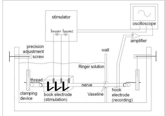
**Fig 4.** Experimental setup, for clarity only the central slot is shown (reproduced with permission).<sup>3</sup>
