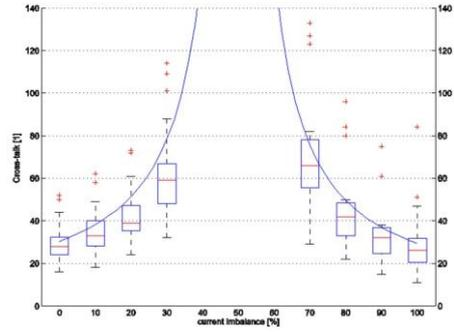
**Fig 7.** Cross-talk ratio depending of current imbalance for Independent between slots, Unpaired, anodes (IP) - Box plot represent measured data from<sup>3</sup> continue line represent simulated data.
