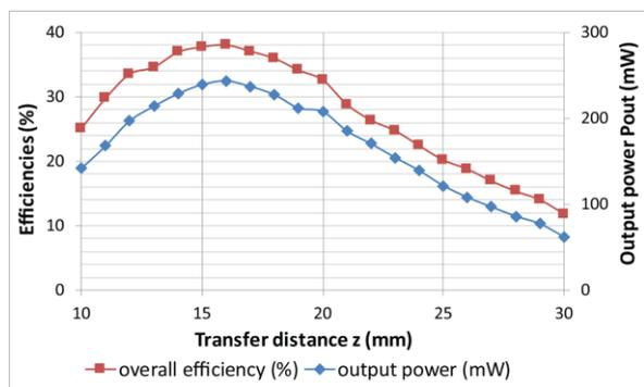
**Fig 5.** System efficiency and output power variation with the transfer distance  $z$ . Supply voltage  $V_{cc}=8V$ ; Rectification diodes forward voltage  $V_{diode}=0.35V$ .
