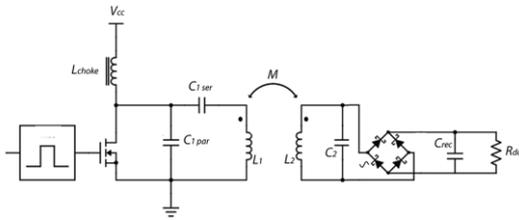
**Fig 3.** Power transfer system PTS obtained at the end of the design methodology for our example.
