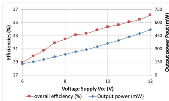
**Fig 6.** System efficiency and the output power variation with the supply voltage. Power transfer distance  $z=21mm$ ; Rectification diodes forward voltage  $V_{diode}=0.35V$ .
