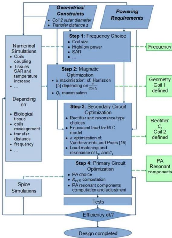
**Fig 1.** Design methodology chart flow presenting the different steps to follow from the initial requirements and constraints to the obtention of an efficient power transfer system, and the possible simulations to perform in parallel in order to improve the analytical and experimental process.
