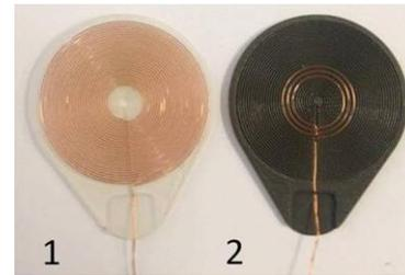
**Fig 2.** Designed Coils where the coil 1 and 2 are respectively the primary and the secondary coils.
