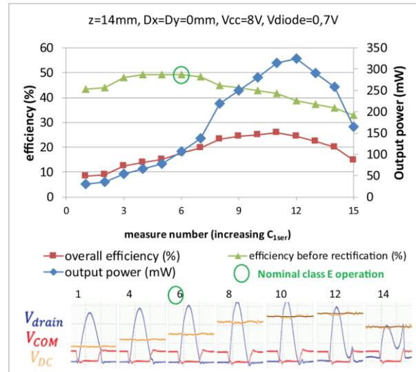
**Fig 4.** Efficiency before and after rectification, output power and screenshots of drain voltage  $V_{drain}$ , gate voltage  $V_{COM}$  and voltage at the load  $V_{DC}$  for different class E power amplifier operating points.
