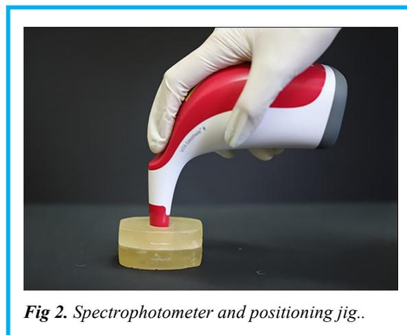
**Fig 2.** Spectrophotometer and positioning jig..
