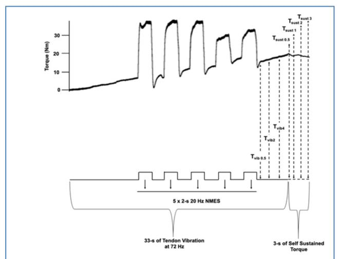
Fig 2. Schematic representation of Tendon vibration superimposed to electrical stimulation protocol to evoke reflexive torque responses.
