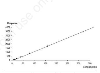
Figure 3. Linear calibration curve of Valproic acid at coentrations from 10 to  $320 \mu g/mL$ .
